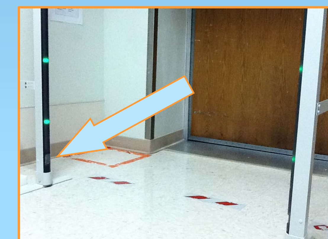
Figure 4. Arrow points at the optical sensor located at the base of the detector.
